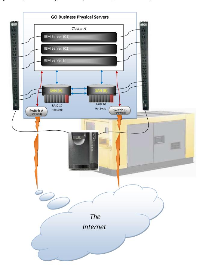
High availability, reliability and performance is further delivered through full redundancy across operating systems, server clustering and real-time mirroring.
